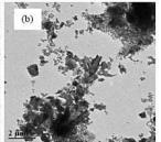
they found that at a lower percentage, the particles were in the form of weak chain-like aggregations as a dense three-dimensional network and were thermally conductive, while for Higher percentages, dense cloud-like accumulations and reduced heat transfer paths are observed.
